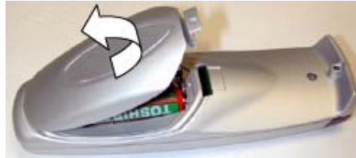
Image 2-6 Battery cover removal
